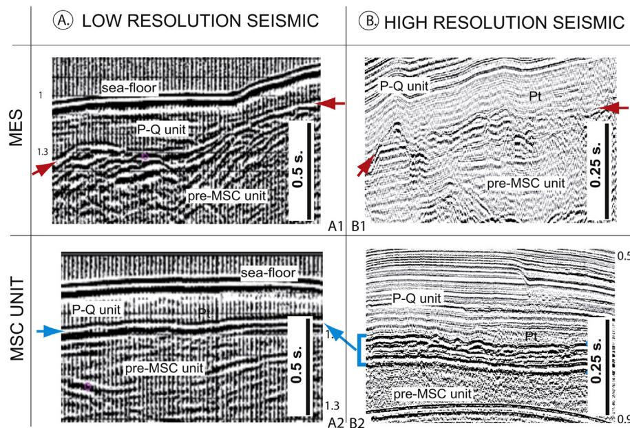
**Figure 6.** Sections showing the different seismic facies of the MSC unit and the MES in the study area, based on the available low-resolution (column A) and high-resolution (column B) seismic data. P–Q unit = Pliocene–Quaternary seismic unit. Pt = transparent seismic facies at the base of the P–Q unit. Red arrows show the MES. In blue: the MSC unit. (For interpretation of the references to colour in this figure legend, the reader is referred to the web version of this article.)
