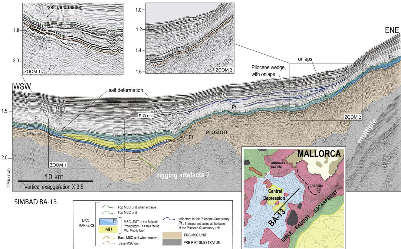
**Figure 11.** Seismic profile Simbad-BA13 in the Mallorca sub-basin illustrating the MSC unit extending from the Central Depression to the Mallorca slope. The MSC unit in the Central Depression contains the MU, which is responsible for salt deformation (Zoom 1), with the thin facies (Ft) on top, which extends onto the borders. In the Mallorca slope domain, the MSC unit thins upwards and the Ft onlaps onto the MSC unit present on the slope (Zoom 2).
