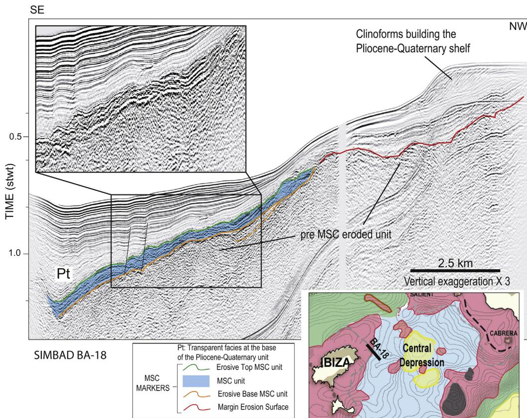
**Figure 10.** Seismic profile Simbad-BA18 in the Mallorca sub-basin illustrating the MSC unit present in the Ibiza slope domain. The MSC unit is present up to 0.6 s TWTT, associated with disturbed seismic facies linked to gliding on its base (Zoom 1). The base of the MSC unit is clearly erosive here. Upslope, the MSC unit thins upwards, onlapping onto the Ibiza margin and passing into the MES.
