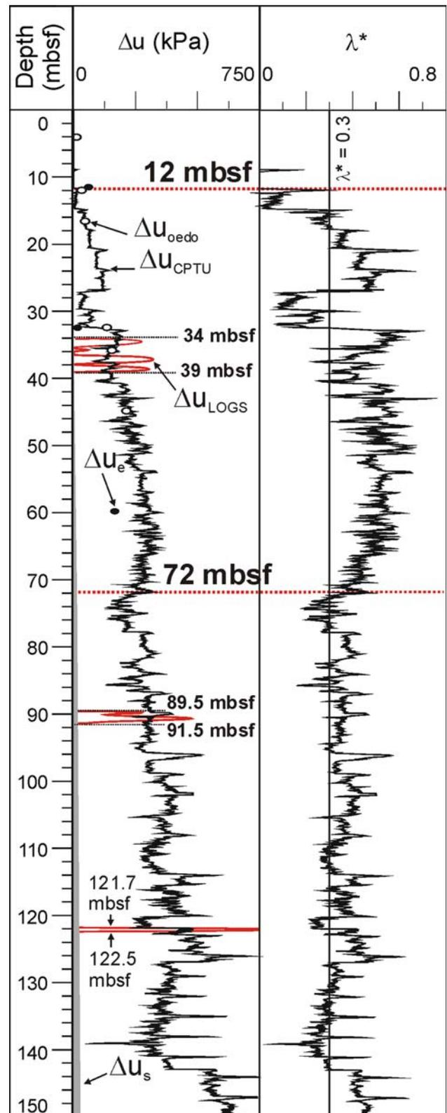
**Fig. 6** Excess pore pressure ( $\Delta u$ ) and overpressure ratio ( $\lambda^*$ ) at PRGL1 site.  $\Delta u_{\text{oedo}}$  measurements are derived from oedometer tests,  $\Delta u_{\text{CPTU}}$  from in situ tests,  $\Delta u_e$  from dissipation tests, and  $\Delta u_{\text{LOGS}}$  from the p-wave downhole logging profile
