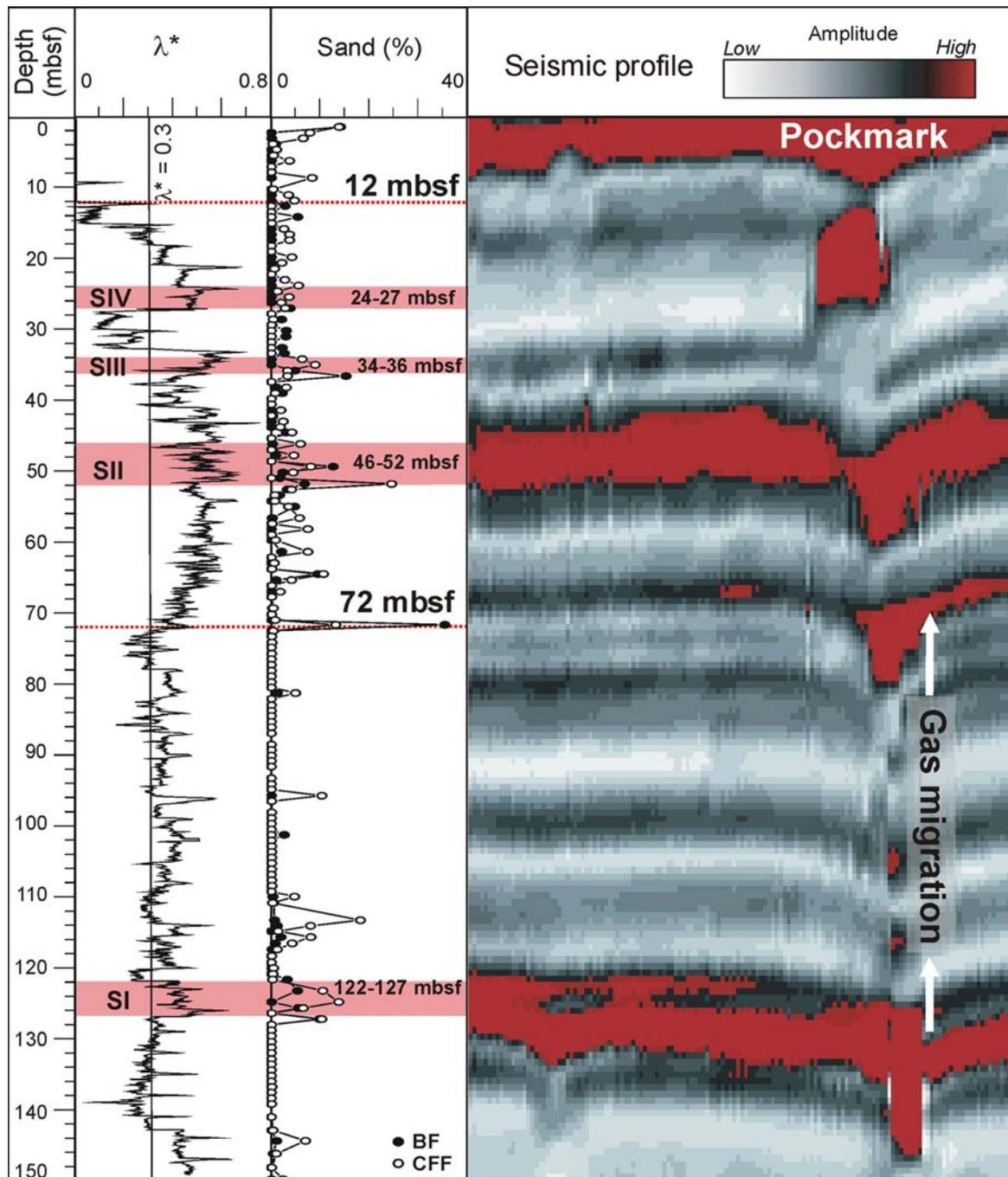
**Fig. 8** Correlation amongst overpressure ratio ( $\lambda^*$ ), sand contents and a seismic reflection profile across site PRGL1 site. Sand contents correspond to both the bulk fraction (BF) and the carbonate free fraction (CFF). Seismic amplitude scale in upper right corner. Pink fringes from 24–27, 34–36, 46–52 and 122–127 mbsf correspond to
