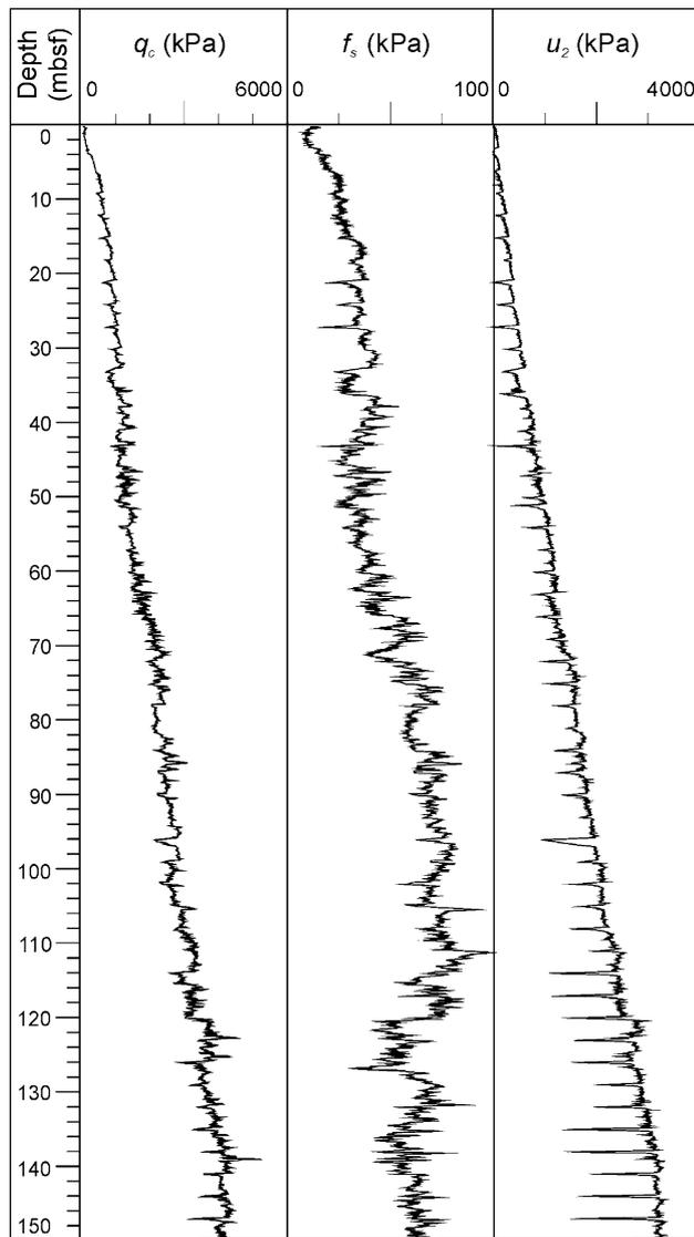
**Fig. 3** CPTU profiles from borehole PRGL1\_3 borehole.  $q_c$  is the cone tip resistance,  $f_s$  is the sleeve friction and  $u_2$  the pore pressure. 3 m spaced  $u_2$  negative peaks are losses in CPTU readings and, therefore, are unrelated to soil type changes
