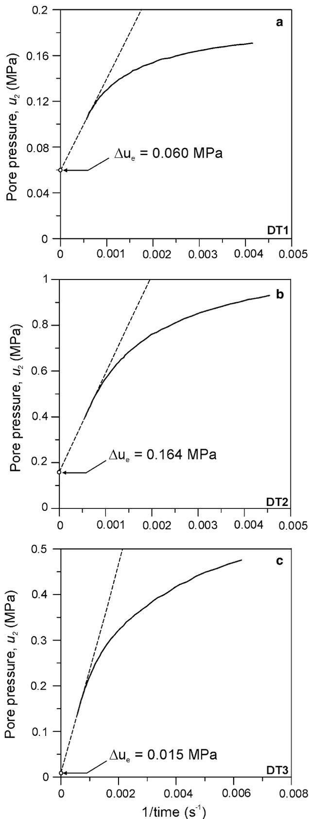
◀ **Fig. 7** Equilibrium pore pressure ( $\Delta u_e$ ) measured during CPTU dissipation tests. **a** Dissipation test DT1 at 11.7 mbsf, **b** dissipation test DT2 at 32.6 mbsf and **c** dissipation test DT3 at 59.9 mbsf
