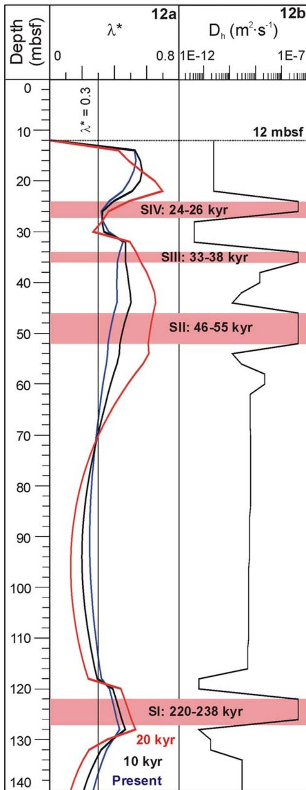
◀ **Fig. 12** Time needed for the dissipation process of the pore pressure during the last sea level rise. **a**  $\lambda^*$  profiles obtained from Eq. (13) (Appendix D.1) and showing excess pore pressure dissipation during the last sea level rise (from 20 kyr to present). **b** The profile of the hydraulic diffusivity used in the calculation based on Eq. (14) (Appendix D.2)
