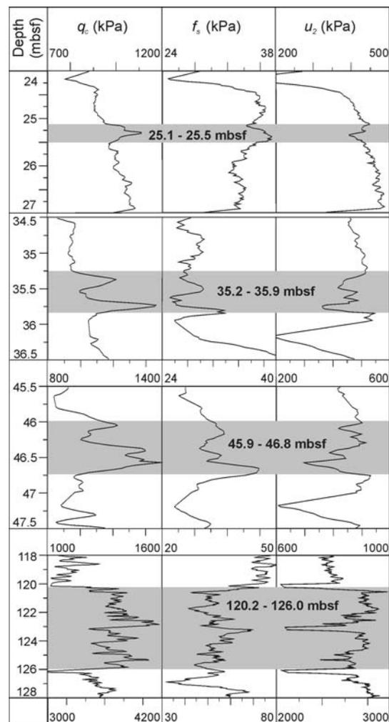
**Fig. 10** CPTU behaviour in the sand-bearing overpressured layers identified. Relative high sand contents (mainly in the CFF, Fig. 8) are characterized by increases in cone resistance ( $q_c$ ) and a reduced pore pressure ( $u_2$ ) due to the permeability of sand
